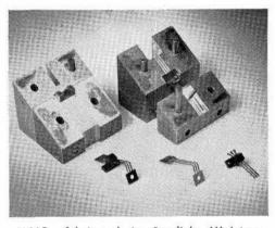
MOLD, fabricated in Sandia's Miniature Machine Shop, allows for precision positioning of electrical contacts for a tiny connector
